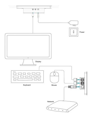
HDMI cable, and connect the mouse, keyboard, and power adapter.
